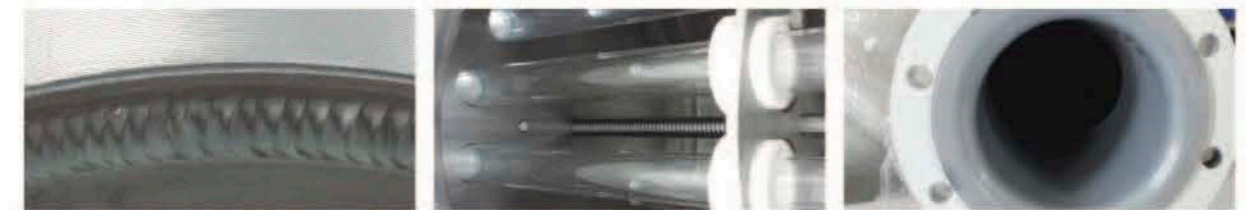
"Fish-scale" external welding
